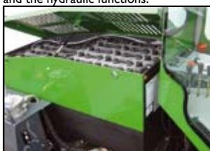
The battery compartment on the C4000 Electric.
